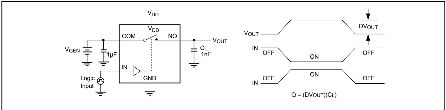
Figure 2. Charge Injection
