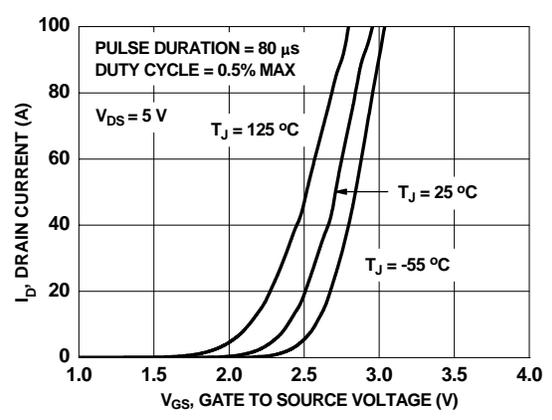
**Figure 5. Transfer Characteristics**
