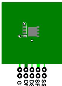
a.  $50^\circ\text{C}/\text{W}$  when mounted on a 1 in<sup>2</sup> pad of 2 oz copper.
