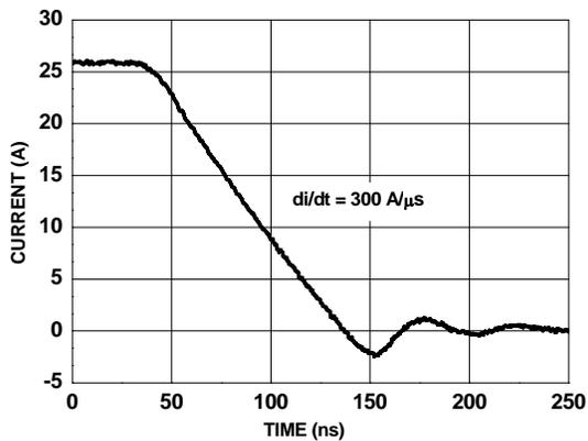
Figure 14. FDMS0306AS SyncFET Body Diode Reverse Recovery Characteristic
