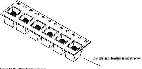
Figure 17. Unit Orientation from reel
