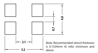
Figure 14. Recommended Soldering Land Pattern
