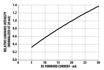
Figure 8. Relative Intensity vs. Forward Current
