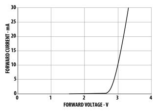
Figure 7. Forward Current vs. Forward Voltage
