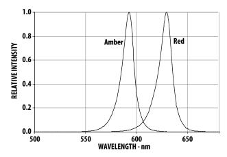
Figure 1. Relative Intensity vs. Wavelength
