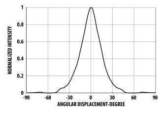
Figure 11a. Radiation Pattern for x-axis
