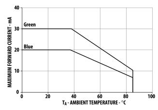
Figure 9. Maximum Forward Current vs. Ambient Temperature
