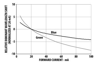
Figure 10. Dominant Wavelength Shift vs. Forward Current
