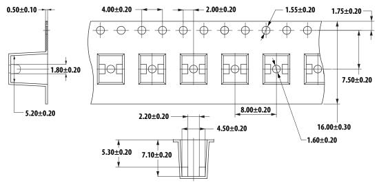
Figure 15. Carrier Tape Dimension
