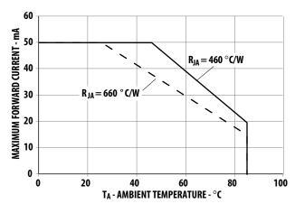
Figure 4. Maximum Forward Current vs. Ambient Temperature
