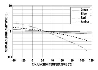
Figure 12. Relative Intensity Shift vs. Junction Temperature
