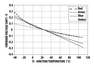
Figure 13. Forward Voltage Shift vs. Junction Temperature
