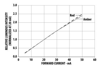
Figure 3. Relative Intensity vs. Forward Current
