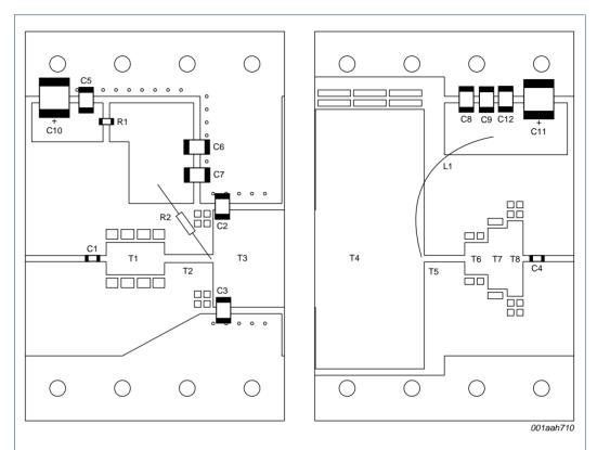
Printed-Circuit Board (PCB): Rogers Duroid 6006;  $\varepsilon_r$  = 6.2 F/m; height = 0.64 mm. See Table 9 for list of components.
