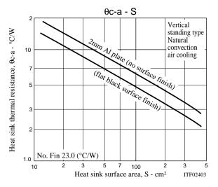
Next we determine the usage conditions with no heat sink by determining the allowable hybrid IC internal average loss from the thermal resistance of the hybrid IC substrate, namely 18.5°C/W.
