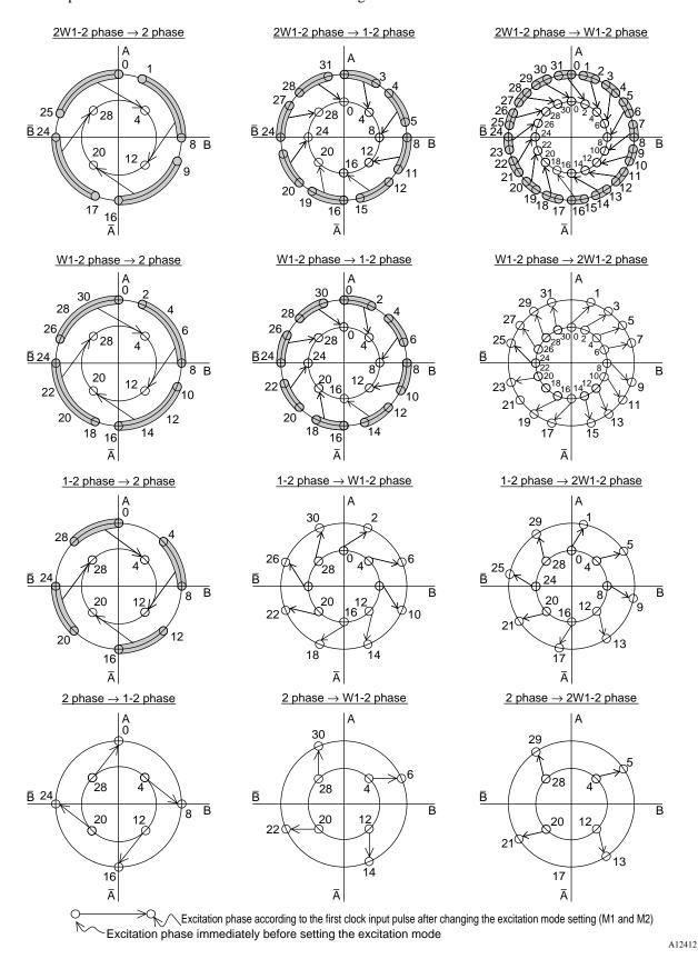
• Excitation phases before and after excitation mode switching <counterclockwise direction>
