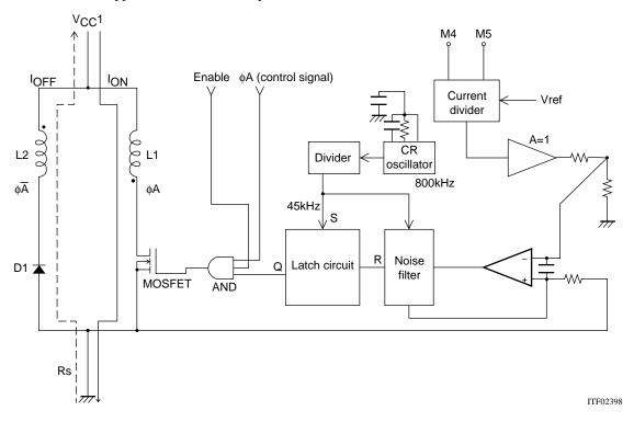
Driver Block Basic Circuit Structure
