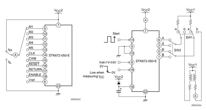
When measuring Ioave: With SW1 set to 'a', Vref = 0.6V When measuring fc: With SW1 set to 'b', Vref = 0V
