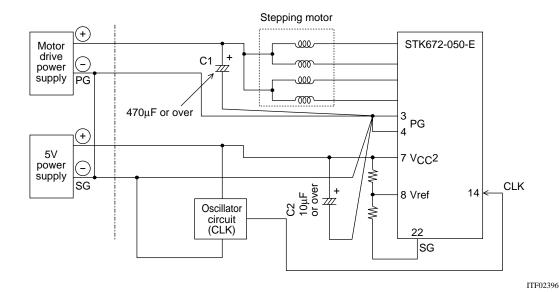
If the grounds for the motor drive supply and the hybrid IC 5V supply are separated:
