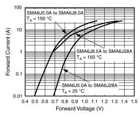
Fig. 5 - Typical Forward Characteristics
