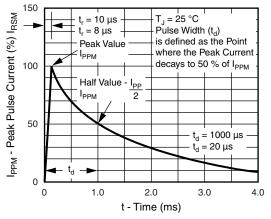
Fig. 3 - Pulse Waveform
