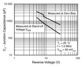
Fig. 4 - Typical Junction Capacitance
