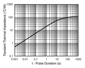
Fig. 6 - Typical Transient Thermal Impedance
