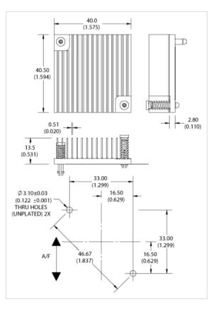
Width: 40.00 Length: 40.50 Height: 13.50 Base Thickness: 2.80 Fin Thickness: Length , Width 0.51 # of Fins: Length , Width 15 Fin Tip to Tip: Finish: AavSHIELD 3C
