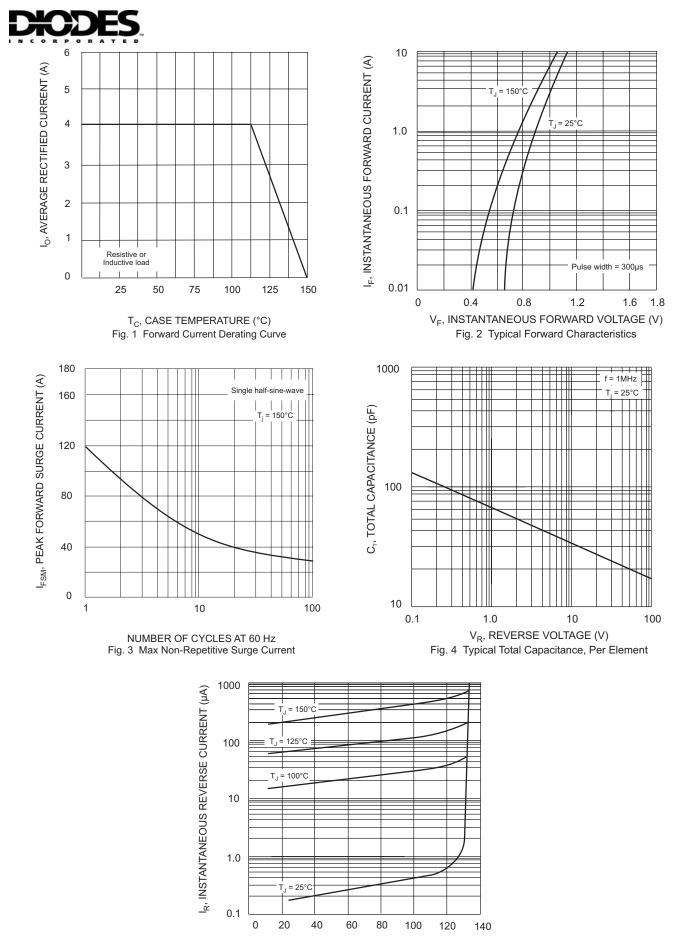
PERCENT OF RATED PEAK REVERSE VOLTAGE (%) Fig. 5 Typical Reverse Characteristics
