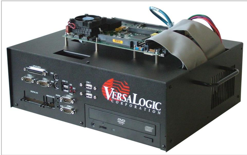
Figure 10. Example EBX Board Installation
