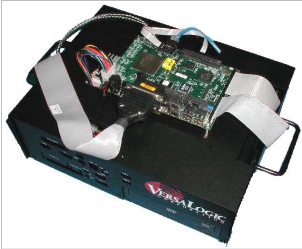
**Figure 11. Example EPIC Board Installation**
