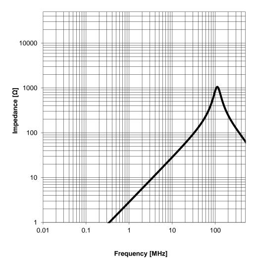
GENERAL TOLERANCE PROJECTION METHOD CREATED CHECKED Würth Elektronik eiSos GmbH & Co. KG EMC & Inductive Solutions KaS BMoe DIN ISO 2768-1m Max-Eyth-Str. 1 74638 Waldenburg **WE-MAIA SMD Power Inductor** Tel. +49 (0) 79 42 945 - 0 ORDER CODE www.we-online.com 784383350047 eiSos@we-online.com DATE (YYYY-MM-DD) BUSINESS UNIT REVISION STATUS PAGE 001.003 Valid 3/7 3015 2017-04-17 eiSos **WÜRTH ELEKTRONİK**
