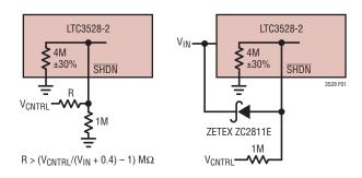
Figure 1. Recommended Shutdown Circuits when Driving  $\overline{\text{SHDN}}$  Above  $V_{\text{IN}}$
