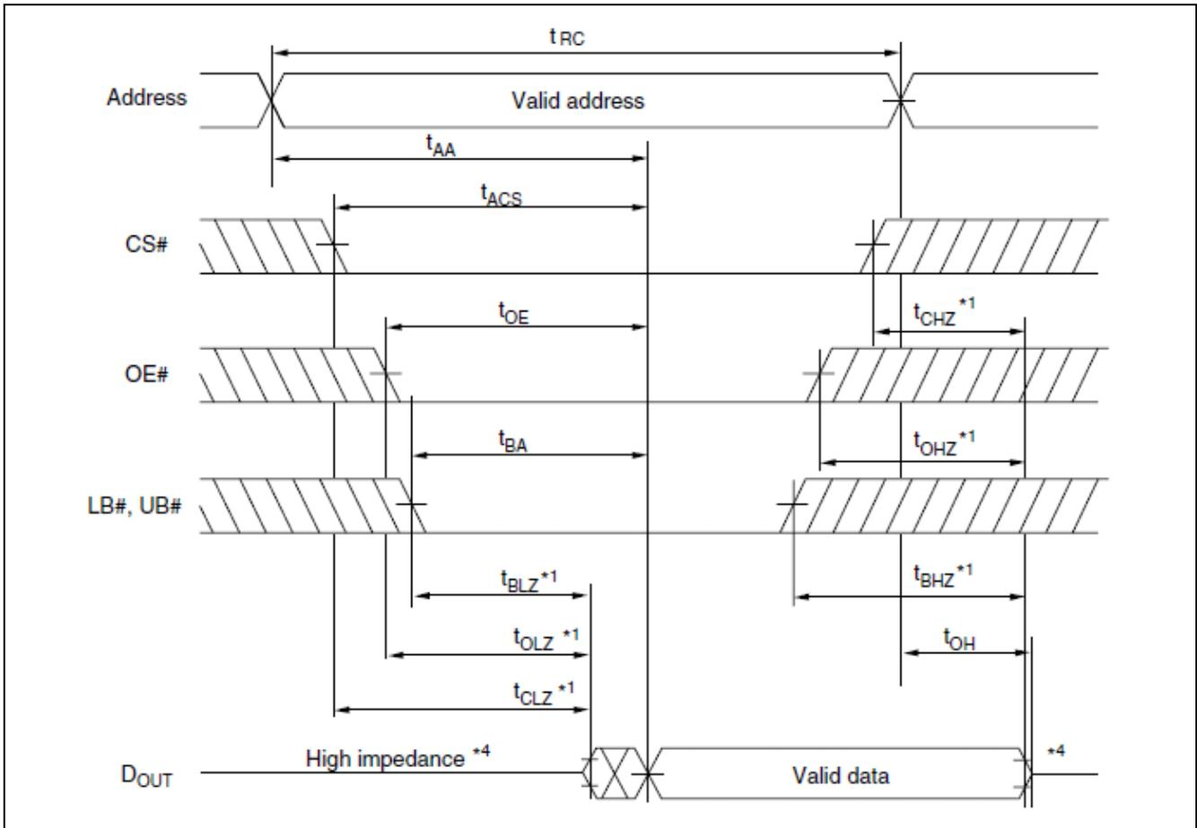
Read Timing Waveform (2) (WE# = V<sub>IH</sub>, LB# = V<sub>IL</sub>, UB# = V<sub>IL</sub>)
