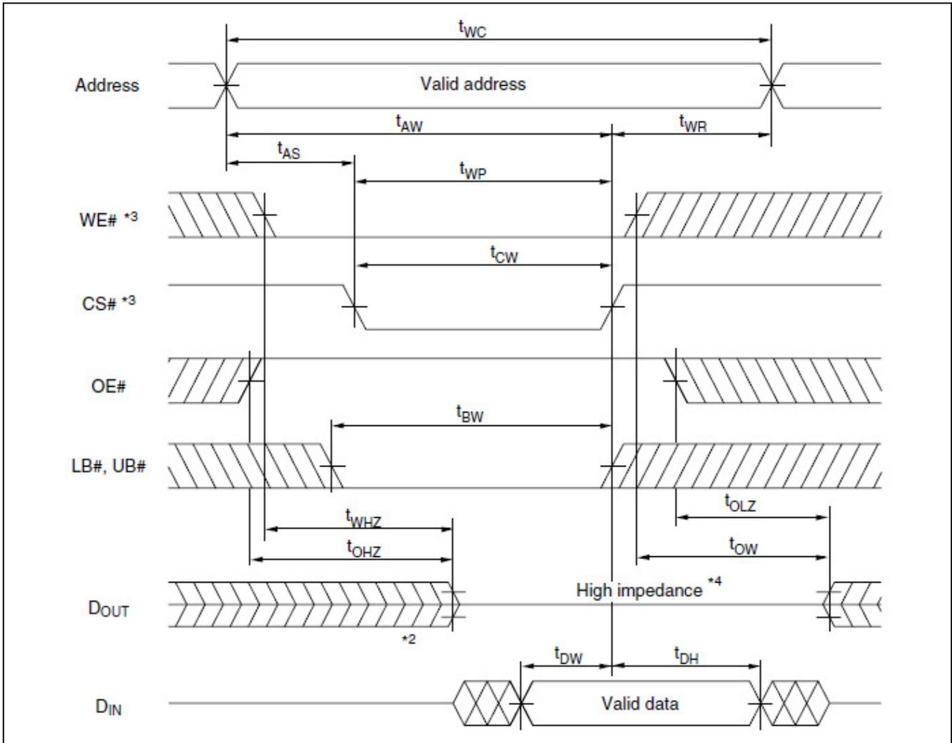
Write Timing Waveform (3) (LB#, UB# Controlled, OE# = V<sub>IH</sub>)
