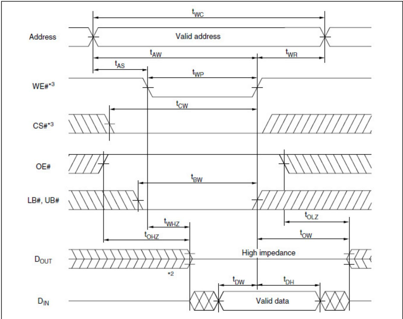
Write Timing Waveform (2) (CS# Controlled)
