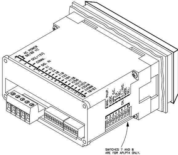
**S1 - ON [MAG.PKUP.]:** Connects a 0.1µf damping input capacitor from input to common. This capacitor is commonly used with magnetic pickup inputs and serves to filter out high frequency noise. It can also be used to filter switch contact closures.
