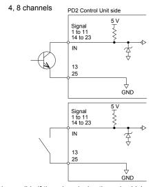
Drive using driver IC or NPN open-collector. Drive is possible if there is a device through which flows an approximately 10 mA current from signal to ground.
