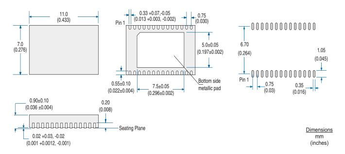
NOTE: Because the metallic pad on the bottom of the DFN package is connected to the substrate of the die, Clare recommends that no printed circuit board traces cross this area to avoid potential shorting issues.
