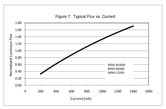
Note for Figure 7: Bridgelux does not recommend driving high power LED Arrays at low currents. Doing so may produce unpredictable results. Pulse width modulation (PWM) is recommended for dimming effects.
