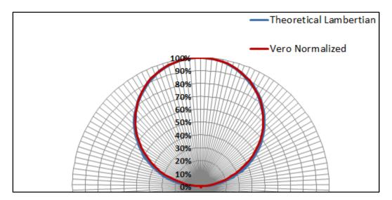
Figure 7: Typical Polar Radiation Pattern
