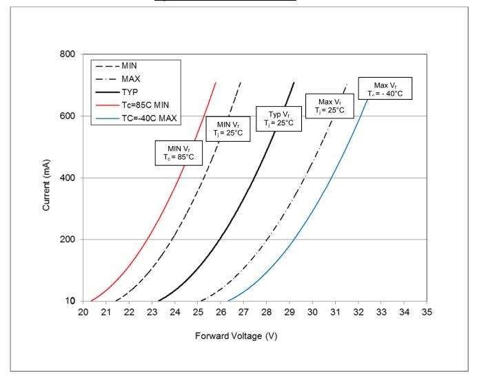
Figure 1: Electrical Characteristics
