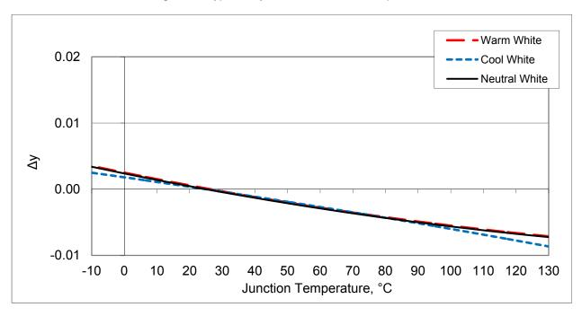
Figure 5: Typical ccx Shift vs. Junction Temperature
