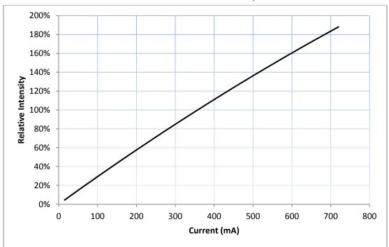
Figure 2: Typical Flux vs. Current,  $T_i = 25$ °C
