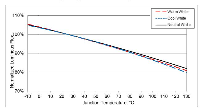
Figure 3: Typical Flux vs. Junction Temperature
