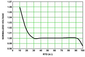
FIGURE 5. TIMING CAPACITOR VOLTAGE vs RTD
