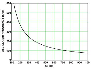
FIGURE 3. CAPACITANCE vs OSCILLATOR FREQUENCY (RTD =  $49.9k\Omega$ )
