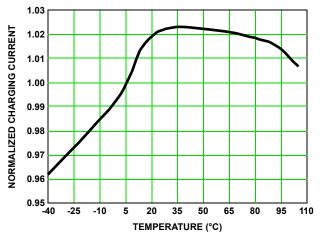
FIGURE 4. CHARGE CURRENT vs TEMPERATURE
