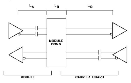
The module transmit and receive insertion loss budgets are different due to the presence of the coupling caps in the module transmit path. The module transmit path insertion loss budget shall be 4.65 dB (3.46 dB + 1.19 dB). The module receive path insertion loss budget shall be 3.46 dB. COM Express connector loss is accounted for separately.
