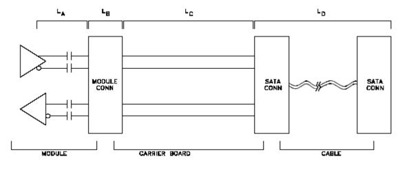
The Serial ATA source specification provides insertion loss figures only for the SATA cable. There are several cable types defined with insertion losses ranging from 6 dB up to 16 dB. Cross talk losses are separate from material losses in the SATA specification.
