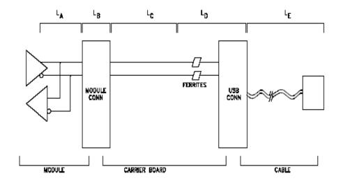
COM Express USB implementations should conform to insertion loss values less than or equal to those shown in the table above. The insertion loss values shown account for frequency dependent material losses only. Cross talk losses are separate from material losses in the USB specification.
