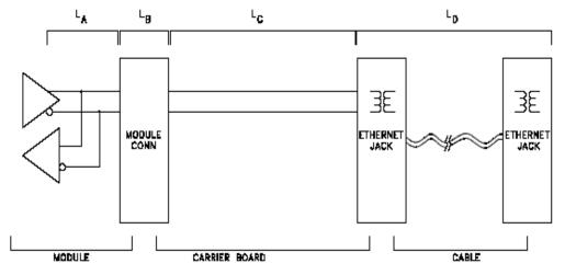
Figure 10: 10/100/1000 Ethernet Insertion Loss Budget
