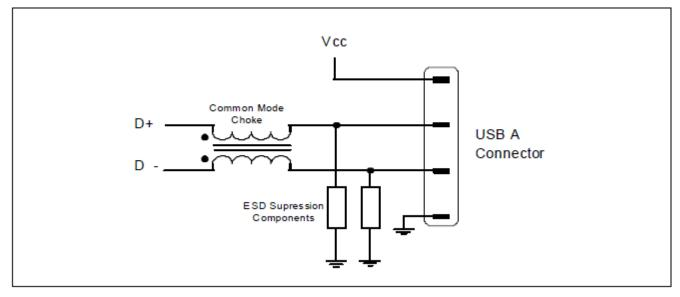
Common mode chokes distort full-speed and high-speed signal quality. As the common mode impedance increases the distortion increases, therefore test the effects of the common mode choke on full speed and high-speed signal quality. Common mode chokes with a target impedance of 80  $\Omega$  to 90  $\Omega$ , at 100 MHz, generally provide adequate noise attenuation.
