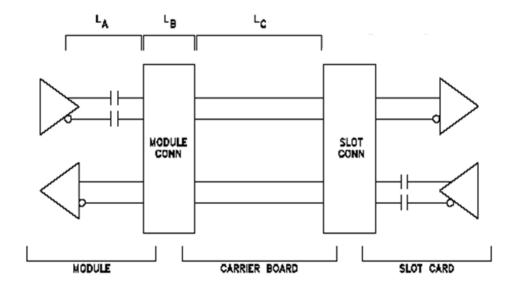
Figure 3: Topology for PCI Express Device Down.
