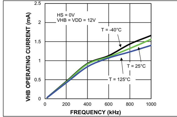
**FIGURE 3-17:**  $V_{HB}$  Operating Current vs. Frequency.
