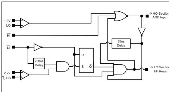
**FIGURE 5-2:** Input Logic Block in Figure 5-1.
