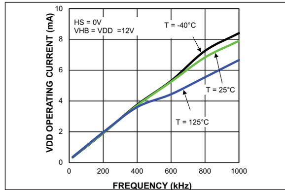
**FIGURE 3-16:**  $V_{DD}$  Operating Current vs. Frequency.
