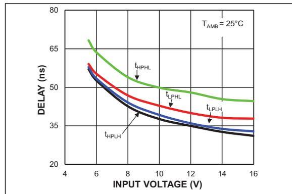
**FIGURE 3-5:** Propagation Delay vs. Input Voltage.
