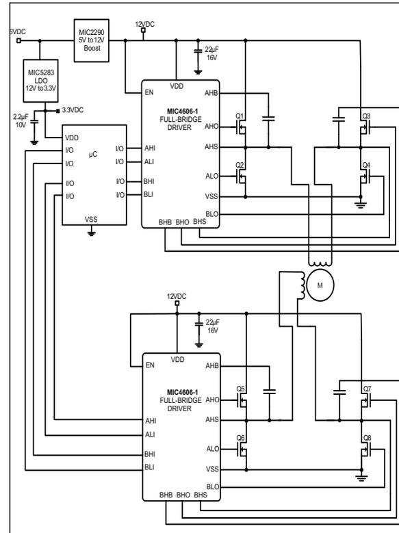
**FIGURE 7-9:** Stepper Motor Driver.
