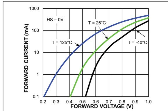
**FIGURE 3-18:** Bootstrap Diode I-V Characteristics.
