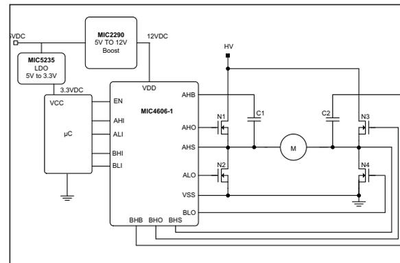
**FIGURE 7-10:** Full-Bridge DC Motor.
