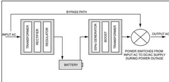
**FIGURE 7-11:** Type I Inverter Topology.
