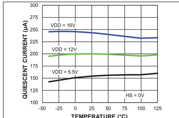
**FIGURE 3-6:**  $V_{DD}$  Quiescent Current vs. Temperature.
