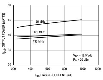
Figure 6. Output Power versus Biasing Current
