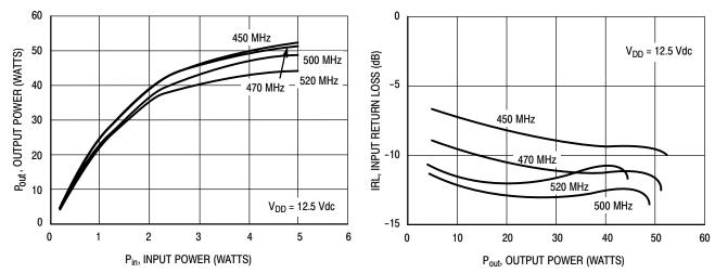
Figure 11. Output Power versus Input Power
