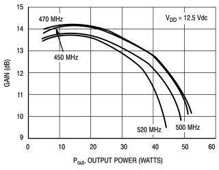
Figure 13. Gain versus Output Power
