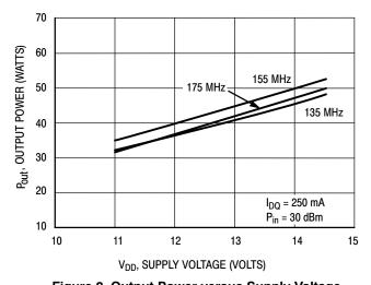
Figure 8. Output Power versus Supply Voltage
