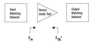
Figure 20. Series Equivalent Input and Output Impedance
