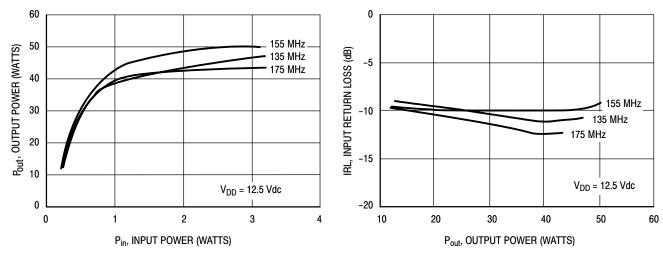
Figure 2. Output Power versus Input Power
