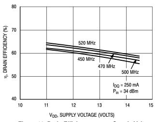
Figure 18. Drain Efficiency versus Supply Voltage
