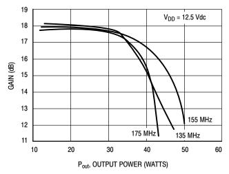
Figure 4. Gain versus Output Power
