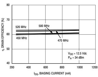
Figure 16. Drain Efficiency versus Biasing Current
