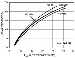
Figure 14. Drain Efficiency versus Output Power
