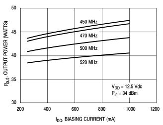
Figure 15. Output Power versus Biasing Current
