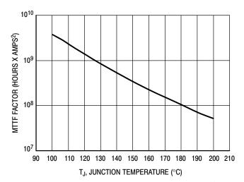
This above graph displays calculated MTTF in hours x ampere<sup>2</sup> drain current. Life tests at elevated temperatures have correlated to better than  $\pm 10\%$  of the theoretical prediction for metal failure. Divide MTTF factor by  $I_D{}^2$  for MTTF in a particular application.
