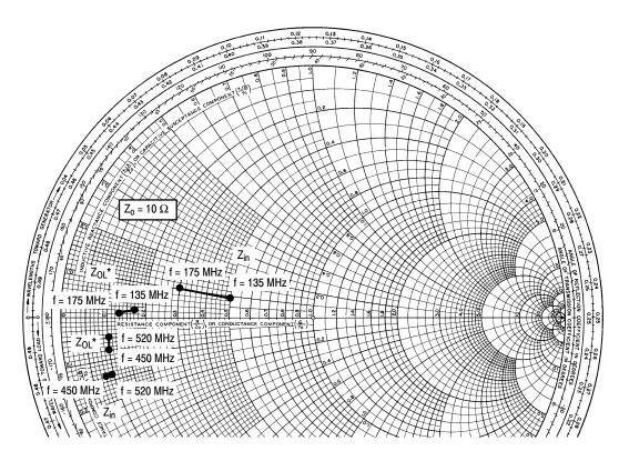
$V_{DD}$  = 12.5 V,  $I_{DQ}$  = 250 mA,  $P_{out}$  = 35 W
