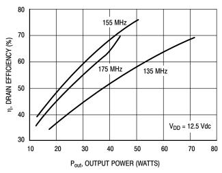
Figure 5. Drain Efficiency versus Output Power
