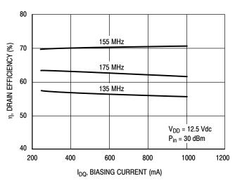
Figure 7. Drain Efficiency versus Biasing Current
