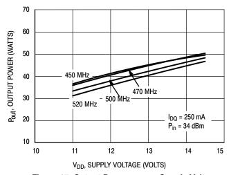
Figure 17. Output Power versus Supply Voltage
