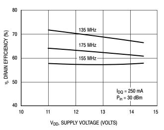
Figure 9. Drain Efficiency versus Supply Voltage
