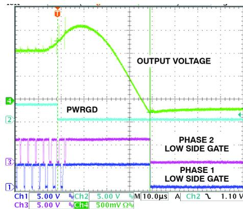
**Figure 40. Overvoltage Protection and Reverse Voltage Protection**
