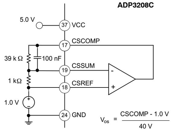
Figure 3. Current Sense Amplifier,  $V_{os}$
