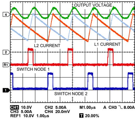
Figure 19. Dual-Phase, Interleaved PWM Waveform, 20 A Load
