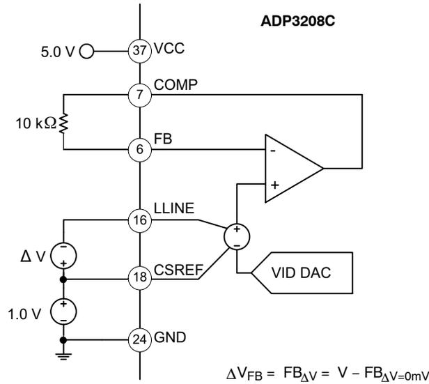
Figure 4. Positioning Accuracy
