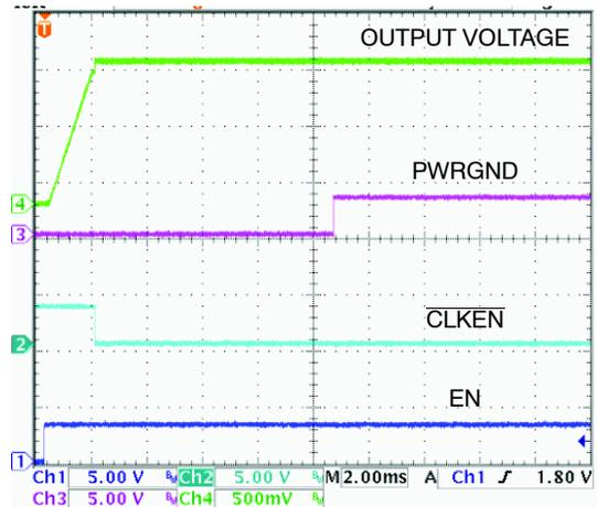
Figure 18. Startup Waveforms
