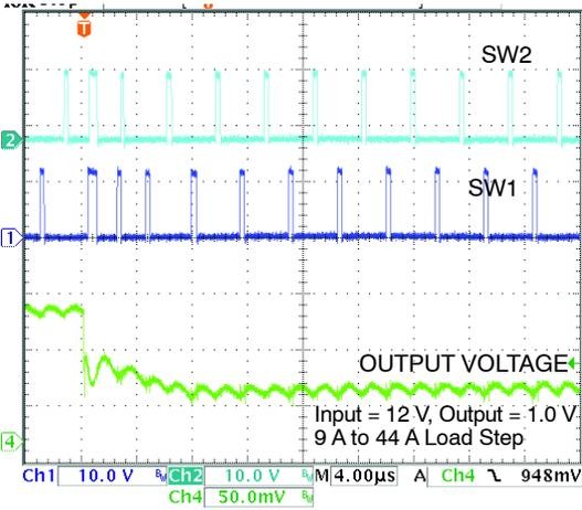
Figure 9. Load Transient with 2 Phases
