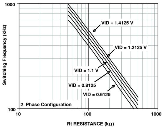
Figure 15. Per Phase Switching Frequency vs. RT Resistance
