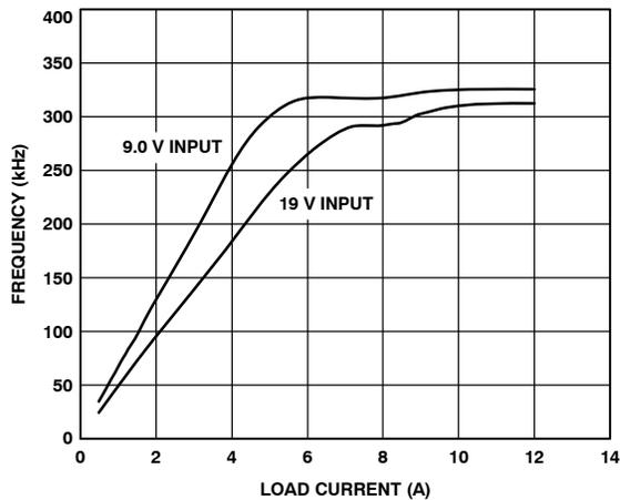
**Figure 39. Single-Phase CCM/DCM Frequency vs. Load Current**
