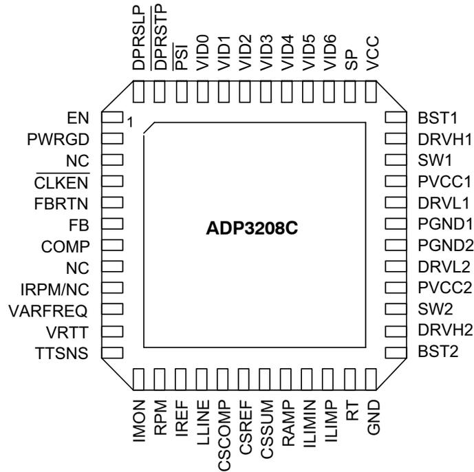
**Figure 5. Pin Configuration**
