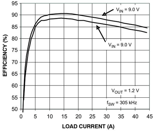
Figure 7. PWM Mode Efficiency vs. Load Current
