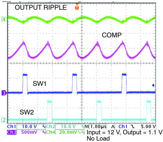
Figure 11. Switching Waveforms in 2-Phase
