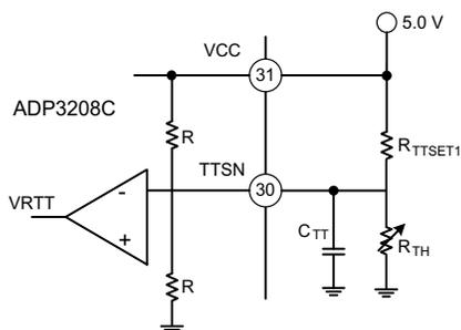
**Figure 45. Single-Point Thermal Monitoring**
