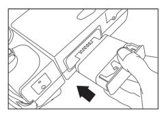
Figure 2. Charge and Insert the Battery
