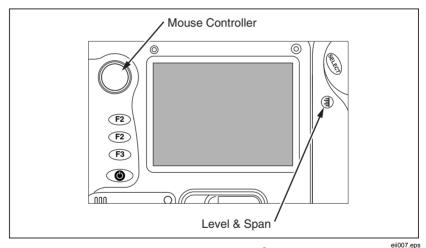
Figure 7. Setting the IR-Fusion<sup>®</sup> Blend Level
