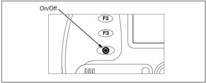
Figure 3. Turning the Power On and Off
