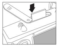
Figure 4. Inserting a Memory Card
