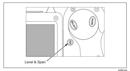
Figure 6. Setting the Level and Span
