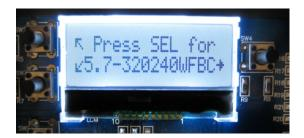
11. When prompted, press the SEL button to continue the demonstration program and scroll through the corresponding files on the SD Card. See Appendix B for SD Card file formatting and editing. You may see a blink on the display as the SD Card is being read and the display is being re-initialized and written.
