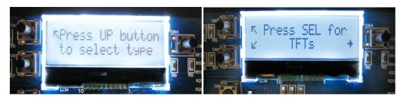
9. The NHDev display will show the first part number model in the selected category. Pressing UP and DOWN buttons will cycle through the available part number models that NHDev is programmed to demonstrate. When the desired part number model is reached, stop pressing buttons.
