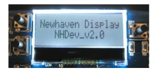
8. The NHDev display will then show "Press UP to select type". Pressing the UP and DOWN buttons will cycle through the available display categories that NHDev is programmed to demonstrate. Pressing the SEL button will enter that category and begin listing specific part number models.
