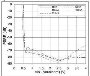
Figure 30. PSRR vs. VIN-VOUT(NOM), VOUT=2.8V
