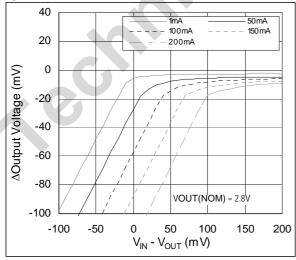
Figure 6. ΔVout vs. Vin; Vout(nom)=2.8V
