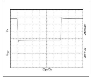
Figure 35. Line Transient Response; IOUT=50mA, VOUT=2.8V, VIN=4.8V to 4.2V
