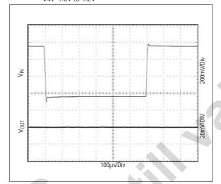
Figure 36. Line Transient Response; IOUT=100mA, VOUT=1.5V, VIN = 3.5V to 2.9V
