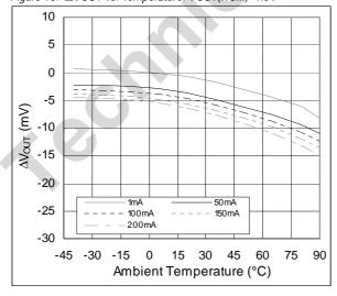
Figure 16. ΔVOUT vs. Temperature; VOUT(NOM)=2.8V
