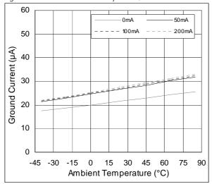
Figure 24. Ground Current vs. Temperature; Vout=2.8V
