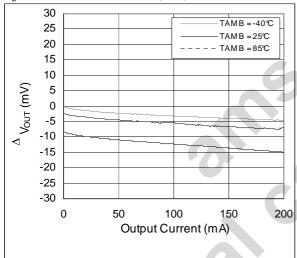
Figure 14. ΔVOUT vs. IOUT; VOUT(NOM)=2.8V
