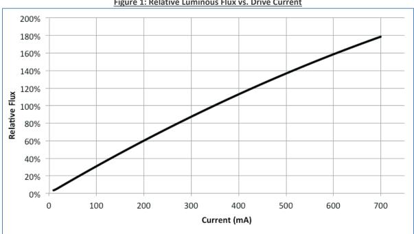
Figure 1: Relative Luminous Flux vs. Drive Current
