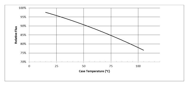
Figure 3: Typical DC ccy Shift vs. Case Temperature
