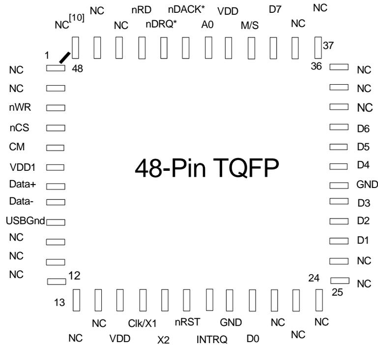
\*See Table 34 on page 22 for Pin and Signal Description for Pins 43 and 44 in Host Mode.
