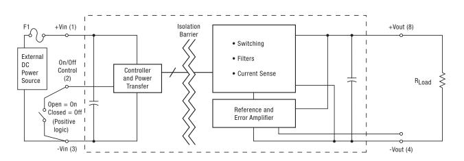
Figure 1. Connection Diagram (without digital interface) Typical topology is shown. Murata Power Solutions recommends an external fuse.
