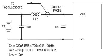
Figure 3. Measuring Input Ripple Current
