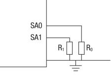
Figure 2. Schematic of Connection of Address Resistors
