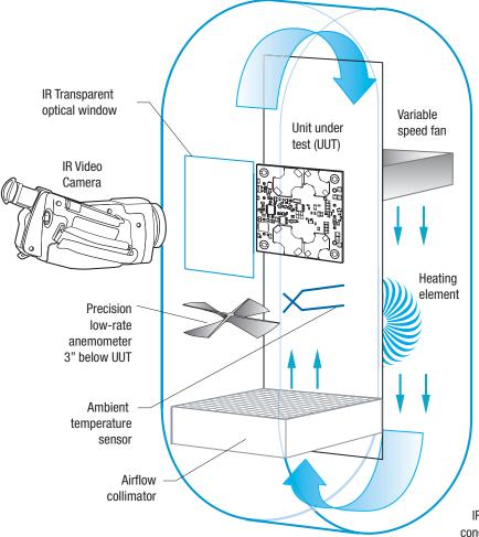
Figure 7. Vertical Wind Tunnel
