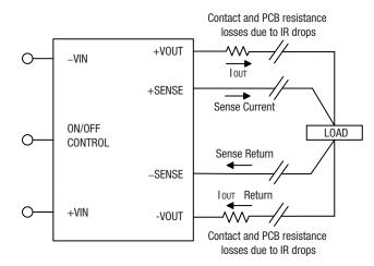
Figure 5. Remote Sense Circuit Configuration
