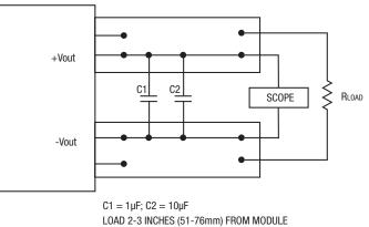
Figure 4. Measuring Output Ripple and Noise (PARD)
