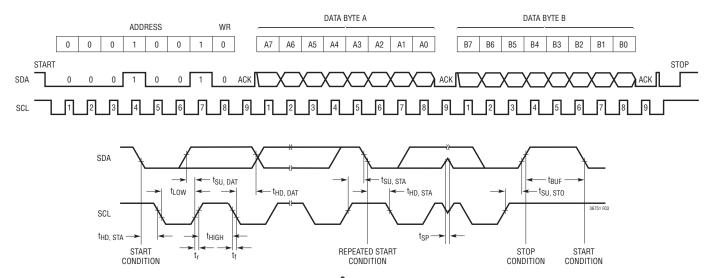
Figure 3. I<sup>2</sup>C Bus Operation
