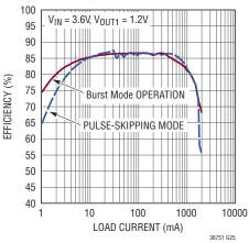
Boost Regulator, Efficiency vs Load
