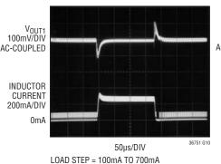
1A Buck Regulators, Transient Response (Burst Mode Operation)
