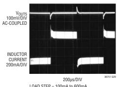
LOAD STEP = 100mA to 600mA  $V_{IN} = 3.6$ V,  $V_{OUT5} = 5$ V
