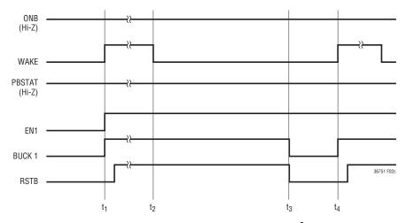
Figure 2c. Power-Up Using an Enable Pin and Power-Down Due to I<sup>2</sup>C Generated Hard Reset
