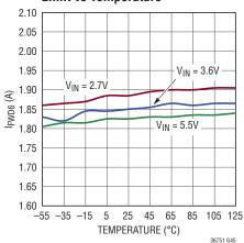
LED Driver, LED Current vs Temperature
