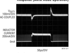
LOAD STEP = 100mA TO 700mA V<sub>IN</sub> = 3.6V, V<sub>OUT1</sub> = 1.2V
