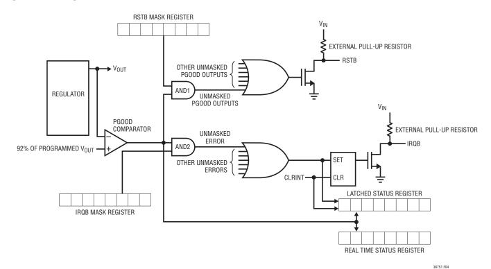
Figure 4. Simplified Schematic Showing RSTB and IRQB Signal Path
