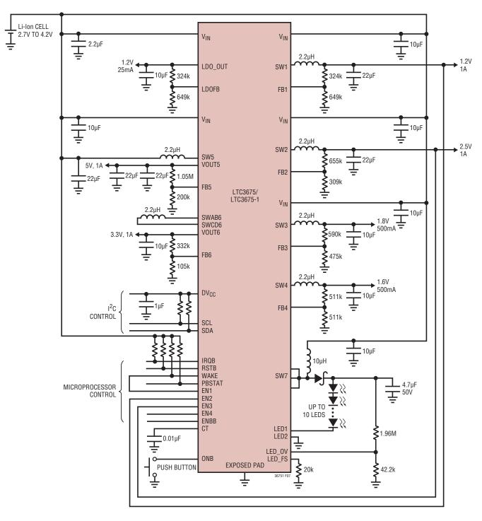
Figure 7. Buck Regulators with Sequenced Start-Up and a Single String of LEDs. Buck Regulators Power-Up in the Sequence Buck1, Buck2 and Buck3
