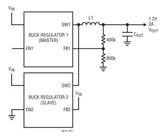
Figure 1. Buck Regulators Configured as Master-Slave
