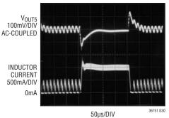
LOAD STEP = 100mA to 600mA V<sub>IN</sub> = 3.6V, V<sub>OUT5</sub> = 5V
