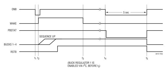
Figure 2b. Power-Up Using WAKE and Power-Down Due to Hard Reset (Sequenced Power-Up, Figure 7)
