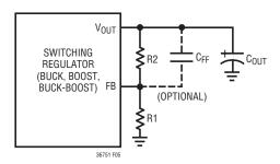
Figure 5. Feedback Components
