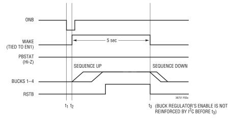
Figure 2a. Power-Up Using WAKE (Sequenced Power-Up, Figure 7)
