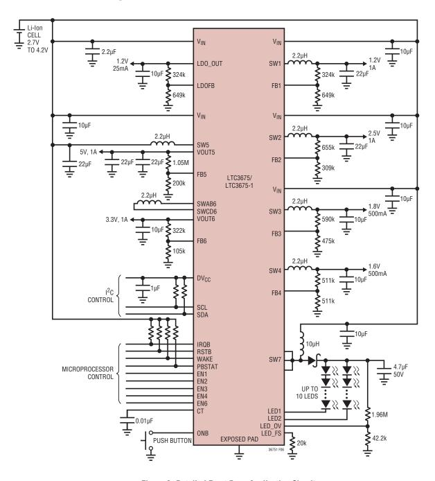
Figure 6. Detailed Front Page Application Circuit
