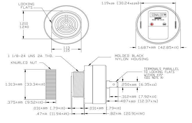
MOUNTING: REMOVE BLACK PLASTIC NUT AND INSERT THREADED FRONT THROUGH 1.25"
