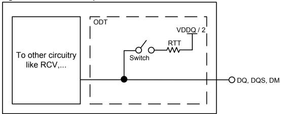
The switch is enabled by the internal ODT control logic, which uses the external ODT pin and other control information. The value of RTT is determined by the settings of Mode Register bits. The ODT pin will be ignored if the Mode Register MR1 and MR2 are programmed to disable ODT and in self-refresh mode.
